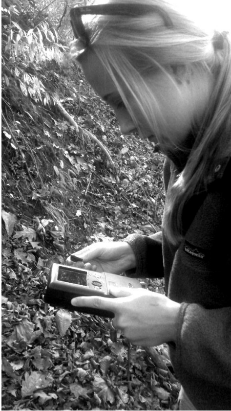
Field assistant Katie Monick replaces data card in a SPYPOINT PRO-X video camera. Photo by Samantha Carpenter
